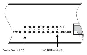
Figure 1-3 Port and Power LEDs
